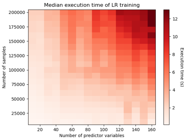
Fig. 2: Median execution times of training the LR model with varying sample sizes and numbers of predictor variables.
