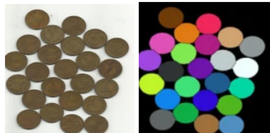
Fig. 2. Visual application of the watershed algorithm on a digital image of coins [4]
